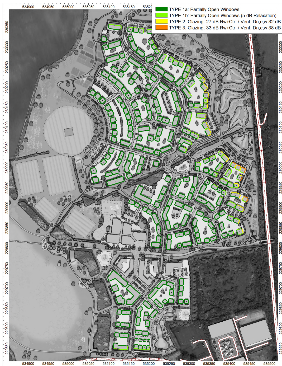
FIGURE 5: OUTLINE FAÇADE SOUND INSULATION PERFORMANCE REQUIREMENTS
